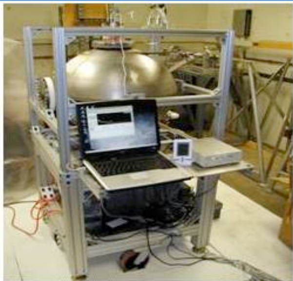
A new reduced-volume manganese bath permits calibration of low-intensity neutron sources a required for DHS applications. (Photograph by: NI&D Group.)
